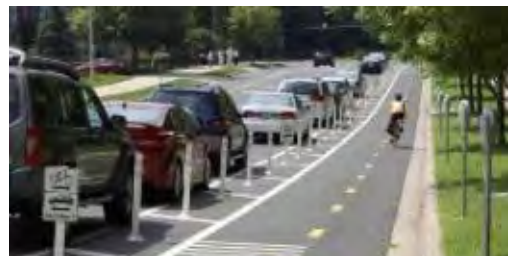
Planned: Parking on north side shifted from curb to add protected bike lanes
