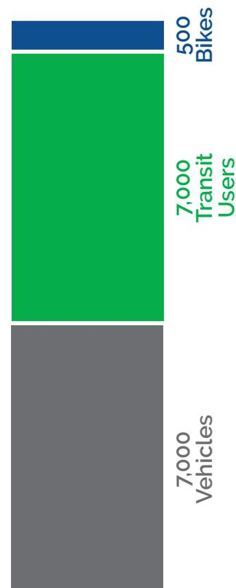
Estimated mode share generated by comparing traffic volumes, transit vehicle load data (2017), and bicycle counts. Daily vehicles were estimated by comparing manual class data from the 2000 block to the 1700 block of Chestnut Street where an AADT figure was available. Bicycle data was estimated using a range of counts from 2010-present and verified against Walnut Street counts. The high variability of bicycle counts (71 - 842) makes this a very generalized estimate.
