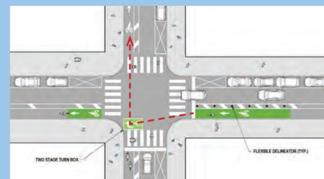
Two-stage turn boxes offer people on bikes a safer way to make turns at cross intersections. Adding these boxes at key locations on Spruce and Pine will give people on bicycles a visible path across the intersection without the need to merge with or cross vehicle traffic.
